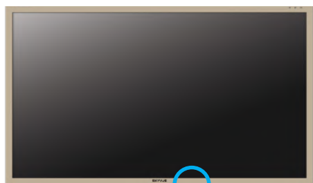
Location of Manual Controls Panel
