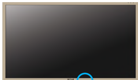
Location of Manual Controls Panel
